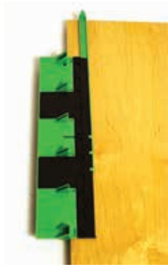
Step 1 Firstly, determine the distance from the top of the door where the first hole is required
