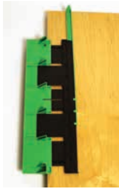
Step 2 Then determine the distance from the side of the door where the first hole is required
