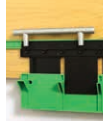
Step 4 For a standard centre, simply off the scale the desired hole centres and mark the door with the position of the second hole
