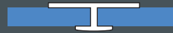
H-Joint Straight panel connector for a series of panels on a flat wall.
