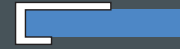
End Cap Used at the vertical open end and when a panel meets the floor.
